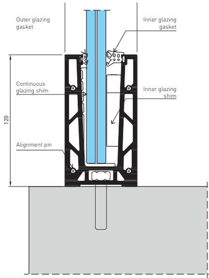
TOP-MOUNTED ON THE SLAB WITH FOOT (ADVANCED)
