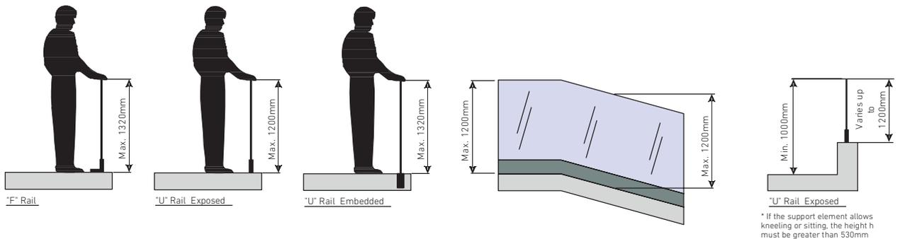
According to the American standard ASTM E 2353-16, E 985-00, the balustrades must be tested with the loads defined for the places and type of use foreseen, namely:
