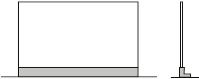
Top-mounted on the slab with foot (advanced)
